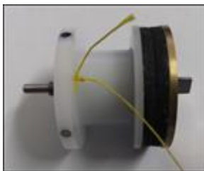
Figure 6-3: BWW Spool String attachment
